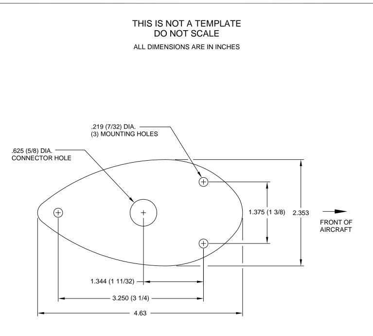
MOUNTING HARDWARE, MOUNTING PAD AND BACK-UP PLATE ARE SUPPLIED WITH ANTENNA
