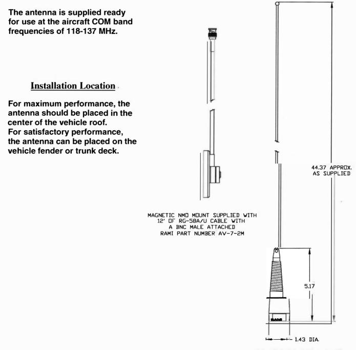
VHF WIDEBAND MOBILE ANTENNA RAMI PART NUMBER AV-7-1A
