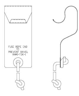
The RAMI-TDK-1 Tie down is used for tying vehicular antenna whips over to prevent damage while traveling of when antenna is not in use.
